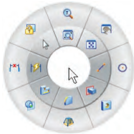
The Radial Menu is sometimes called the Marking Menu. It appears when you hold down RMB. This can be customized for each environment: Sketch, Part, Assembly and Drawing.
