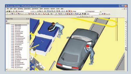
Process Simulate enables manufacturers to virtually develop and verify process plans for their plant's manufacturing systems in a 3D collaborative environment that can be shared by multiple engineering and manufacturing disciplines. Process Simulate is a major component in two Tecnomatix solutions:
